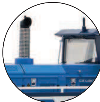
Exhaust pipe panelling made from photo-etched
